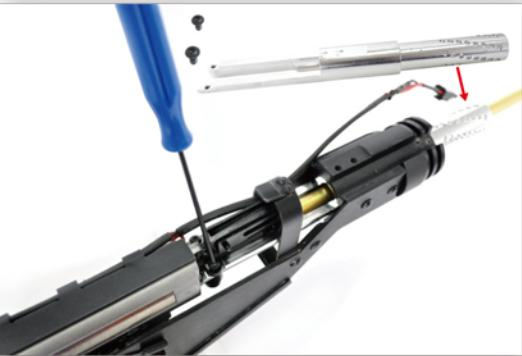
**2. Fix the GearBox Screw, Fix the Fire Selector Plate.**
