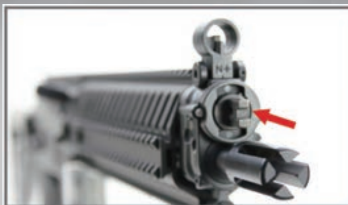
2. Take out the dummy gas regulator.
