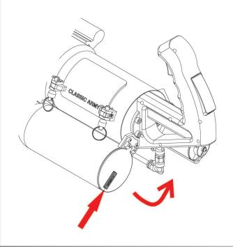
2.Insert the gas bottle to the botton and tight clockwise quickly.
