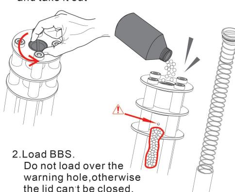
3. Press the spring into the tube and insert it, into the slot and tight it clockwise.
