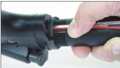
The wire should be held down tightly within the wire path when taking the wire.
