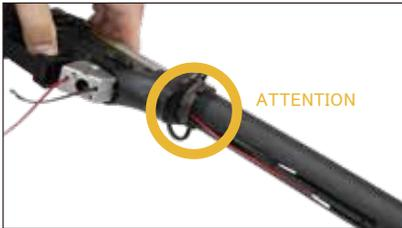
The red line indicates an area where the wire can be damage, please use caution in this area.
