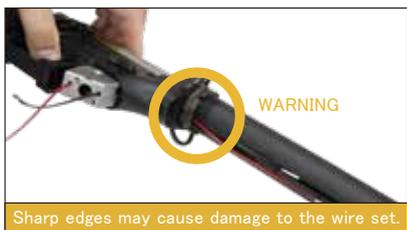
Sharp edges may cause damage to the wire set.
