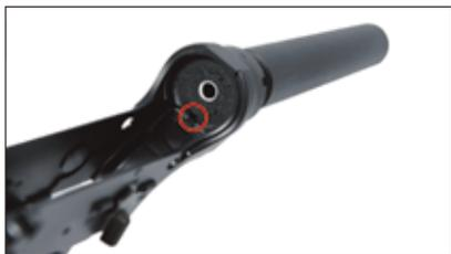
The wire set goes through the circled area indicated on the lower receiver below.
