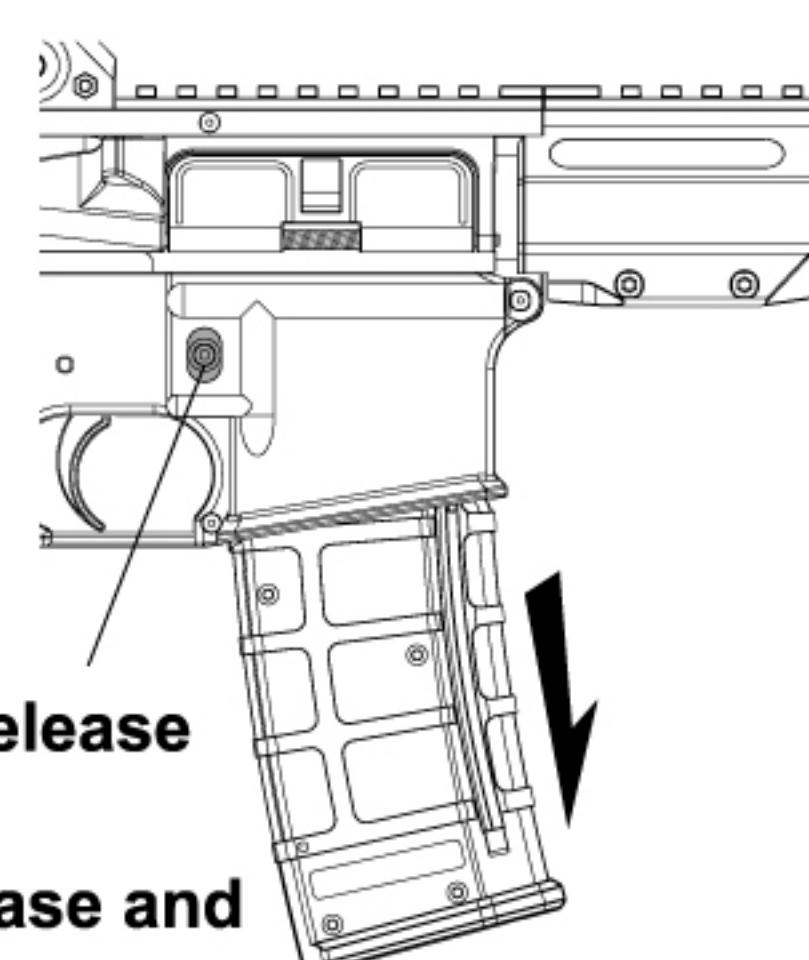
\*Press magazine release and remove magazine
