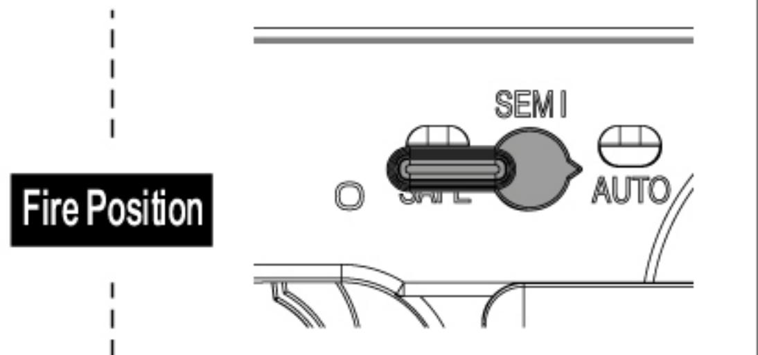
\* When the gun is in safe, the trigger cannot be pulled. Do not force the trigger.
