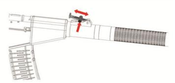
Set the rear sight for desired elevation by pressing the button and move the indicator forwards and backwards along the slide bar.
