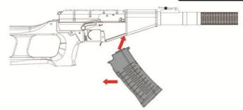
Insert the lug on front of the magazine into the magwell slot, then pull the magazine towards trigger until it snaps into place.
