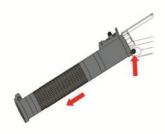
Press the button indicated by arrow then separate the silencer from the rifle in the direction as the arrow shown.
