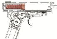
After dry-firing 3-5 shots in semi-auto mode, the piston will complete the shooting cycle and going back to the original position therefore the spring is not being compressed.
