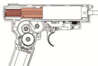
In this situation, the piston is stopped in the middle of the shooting cycle. The spring is now being compressed and it will cause damage to the spring in long run.
