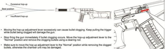
The hop-up adjustment lever behind the ornament plate will be seen when the bolt handle being pulled backward, user can adjust the hop-up by moving the hop-up adjustment lever forwards and backwards.
