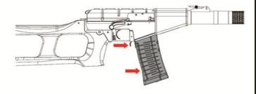
Remove the magazine by pressing the magazine catch towards the magazine, then swing the magazine forwards out of the receiver.
