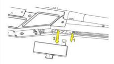
First, remove the magazine by pressing the mag release button. Make sure there is no bullet left inside the rifle.
