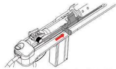
Then release the charging slide, safety off and pull the trigger when ready to fire the rifle. The charging slide will be cycled automatically.
