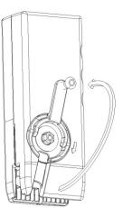
Pivot the crank arm into the "open" position.
