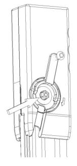
Some magazines have stiffer springs than industry standard, and might require the adjustment of the clutch nut. If your magazines are not getting fully loaded, locate the clutch nut on your M12 Sidewinder, and using a 10mm wrench, rotate it clockwise 1/8 turn, and attempt to load the magazine again. Repeat this step until the M12 loads your magazine completely.
